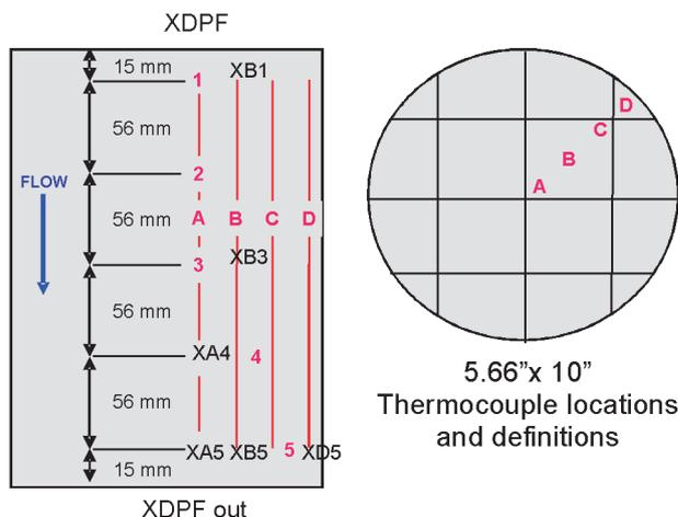
Fig. 2. Thermocouples locations in DPF
