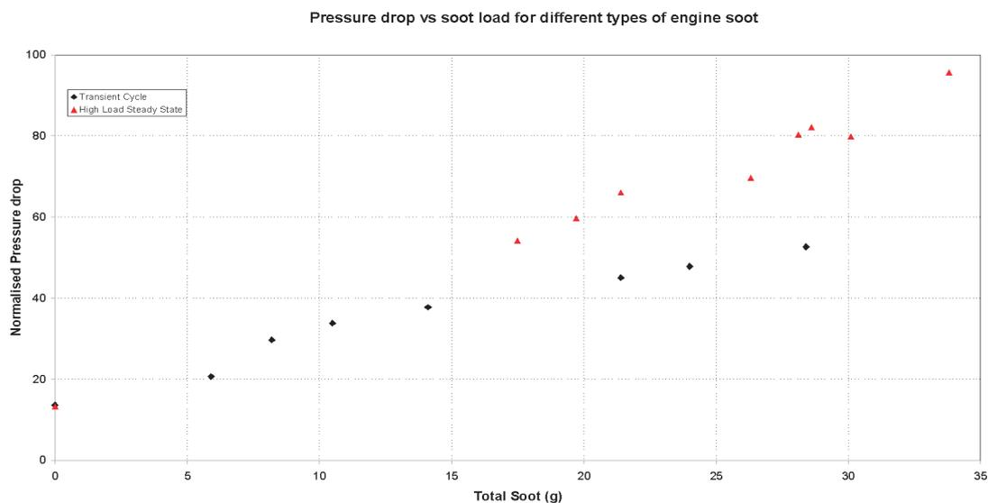
**Fig. 10.** DP vs sootlad for 2 types of Diesel engine soot
