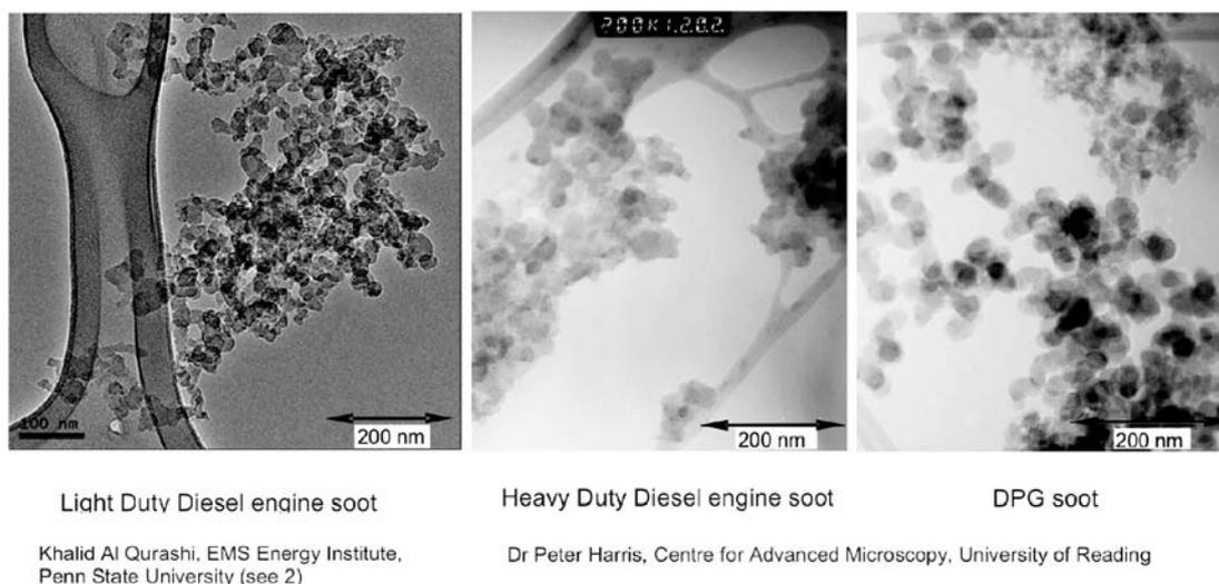
Fig. 11. TEM images of DPG soot and engine soot
