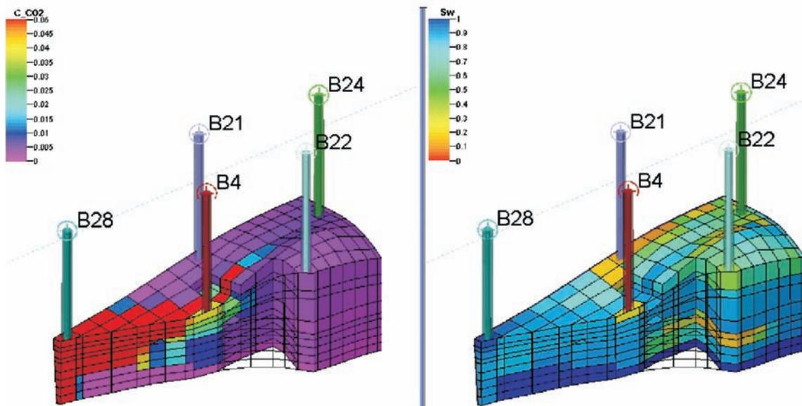
Fig. 12. CO<sub>2</sub> (left panel) and water (right panel) distribution in the Borzęcin structure
