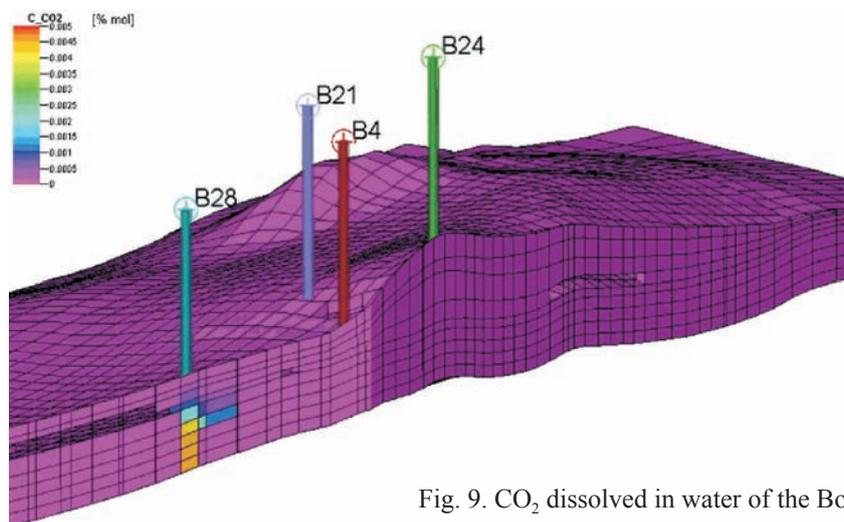
Fig. 9. CO<sub>2</sub> dissolved in water of the Borzęcin structure
