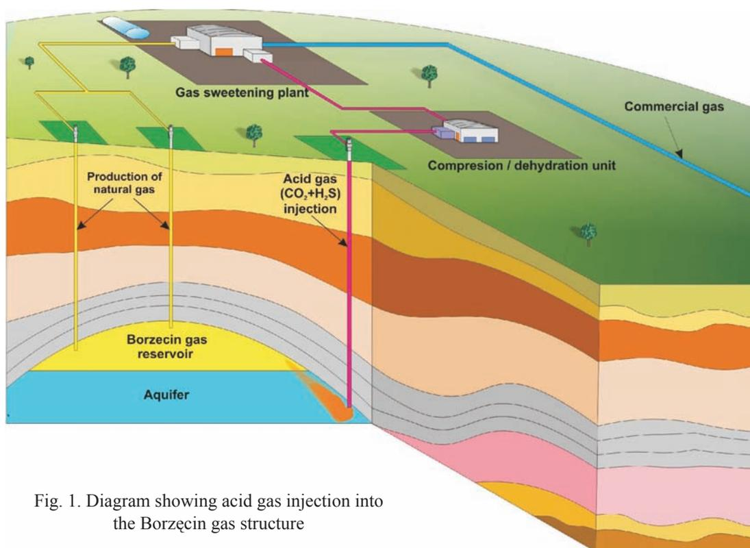
Fig. 1. Diagram showing acid gas injection into the Borzęcin gas structure
