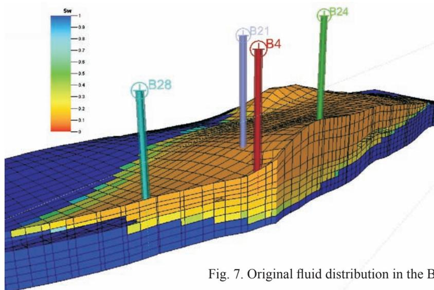
Fig. 7. Original fluid distribution in the Borzęcin structure
