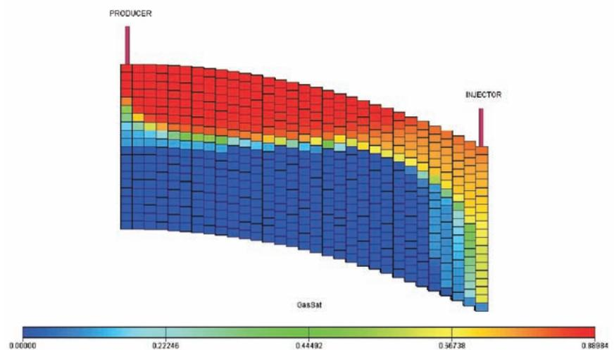
Fig. 6. Gas saturation between injector and producer
