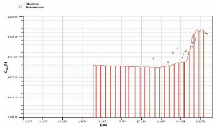
Fig. 4. Example of CO<sub>2</sub> concentration fit for well B-22
