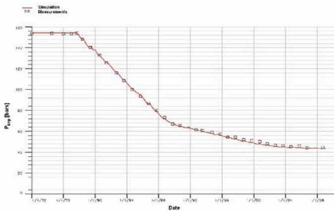
Fig. 3. Example of bottom hole pressure fit for well B-4
