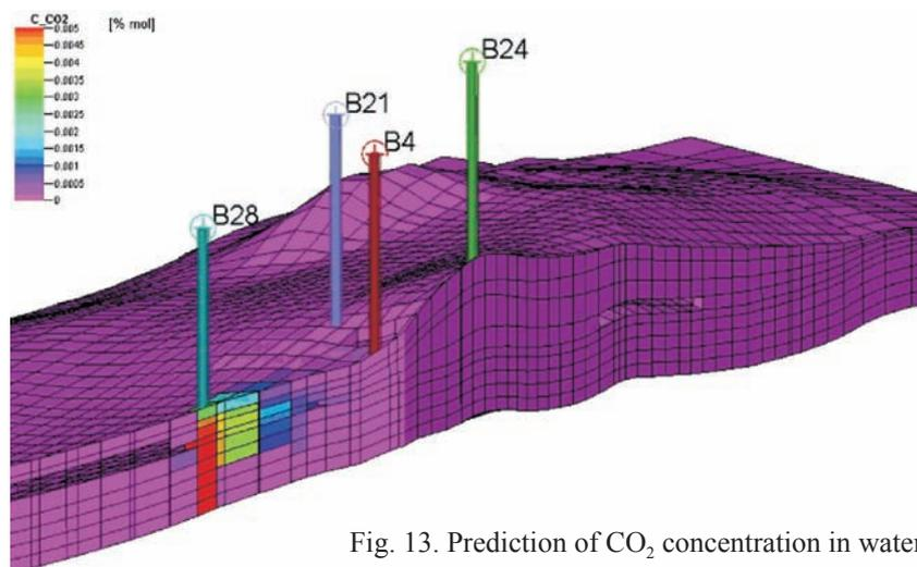
Fig. 13. Prediction of CO<sub>2</sub> concentration in water of the Borzęcin structure
