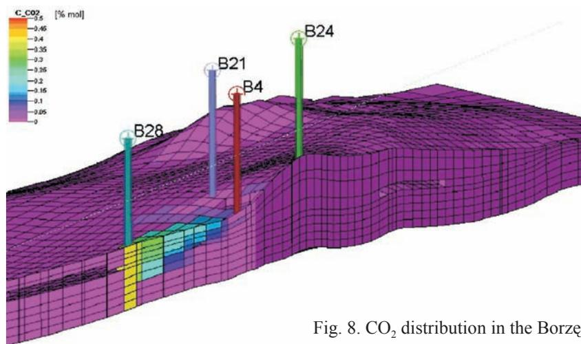
Fig. 8. CO<sub>2</sub> distribution in the Borzęcin structure
