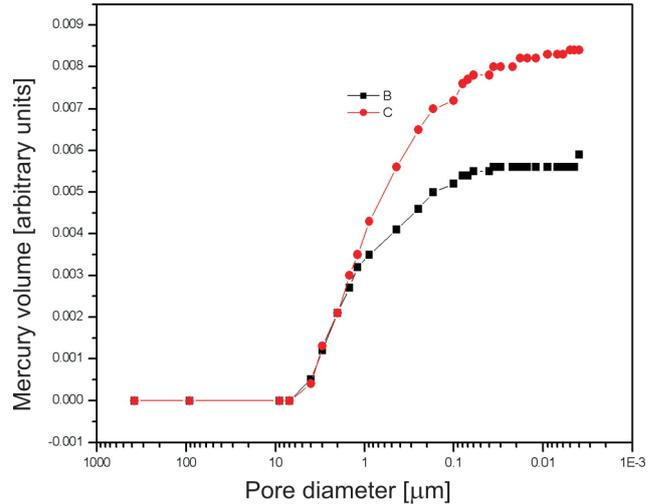
Fig. 7. Cumulative curves for sample "B": B – no crumbled, C – grains 0,5÷1 μm
