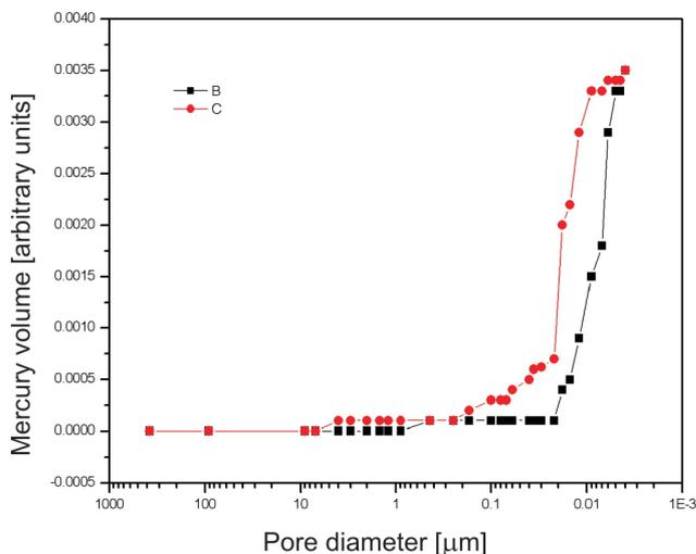
Fig. 2. Pore diameter cumulative curves (sample “C”): B – non crumbled sample, C – crumbled sample (granulation  $1 \div 3 \mu\text{m}$ )
