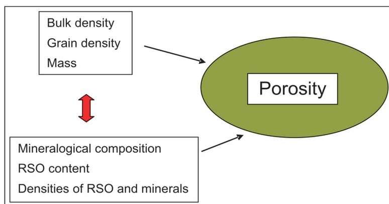
Fig. 1. Sketch of measuring and verifying of porosity
