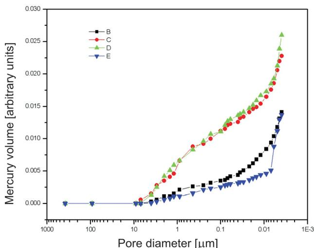
Fig. 3. Pore diameter cumulative curves (sample “A”) for: B – non crumbled sample, C&D – crumbled samples (granulation  $0.5 \div 1 \mu\text{m}$ ), E – crumbled sample (granulation ( $1 \div 3 \mu\text{m}$ ))
