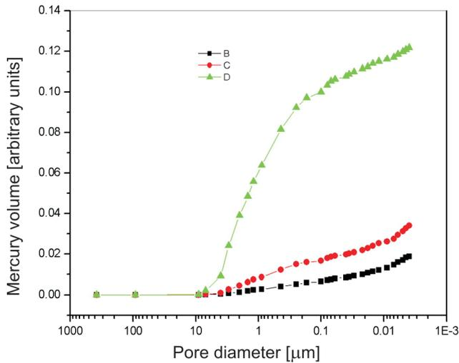
Fig. 4. Pore diameter cumulative curves (sample #2) for: B – non crumbled sample, C – crumbled sample (0.5÷1 μm), D – powdered sample
