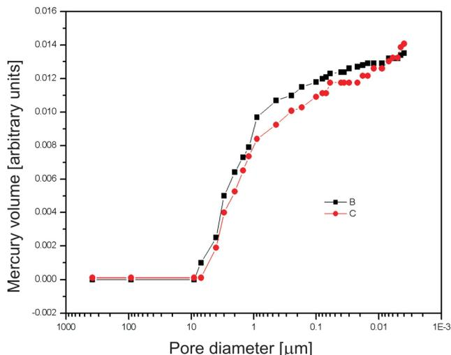
Fig. 9. Cumulative curves for porous and permeable sample (sample "D"): B – no crumbled, C – 0.5÷1 μm grains
