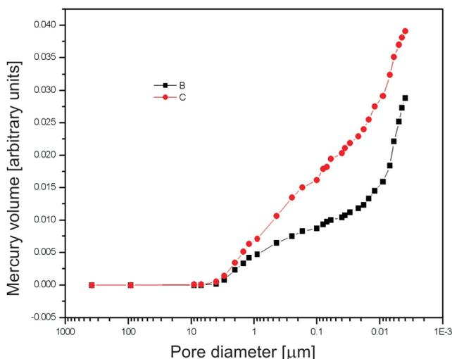
Fig. 6. Pore diameter cumulative curve (sample #4): B – non crumbled sample, C – crumbled sample (0.5÷1 μm)
