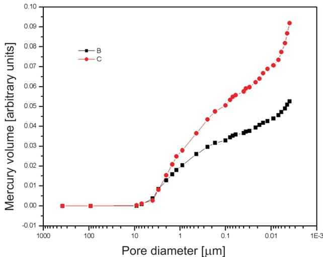
Fig. 5. Pore diameter cumulative curves (sample #3): B – non crumbled sample, C – crumbled sample (0.5÷1 μm)
