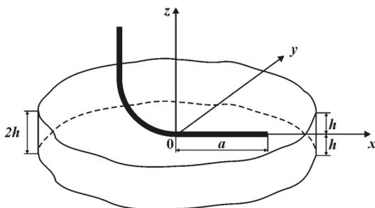
Fig. 5. The horizontal borehole in a productive layer
