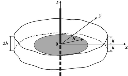
Fig. 3. Illustrative diagram of the horizontal fracture
