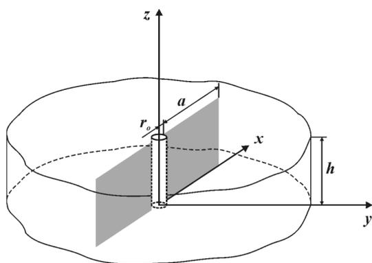
Fig. 1. The borehole with a vertical fracture
