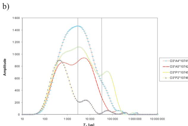
Fig. 3. Distribution of  $T_2$  transverse relaxation time for samples from O-3 well
