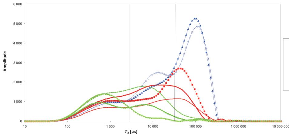
Fig. 5. Model distribution  $T_2$  transverse relaxation time curves, belonging to individual groups Group I (having good reservoir properties) – navy blue, group II (having weak reservoir properties) – red, group III (having poor reservoir properties) – green
