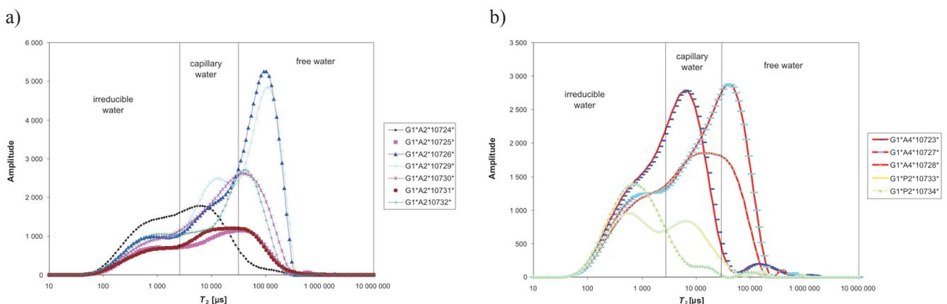
Fig. 2.  $T_2$  transverse relaxation time distributions for samples from G-1 well
