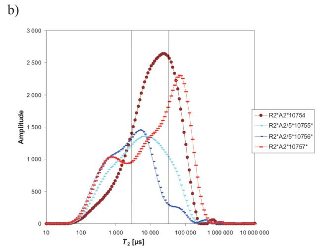
Fig. 4. Distributions of  $T_2$  transverse relaxation time for rock samples from R region
