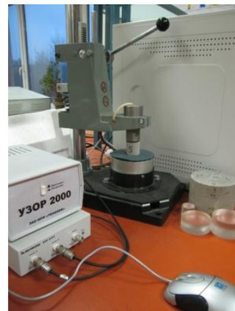
Fig. 1. The device «Uzor 2000» for measuring of ultrasound wave velocity through a porous material
