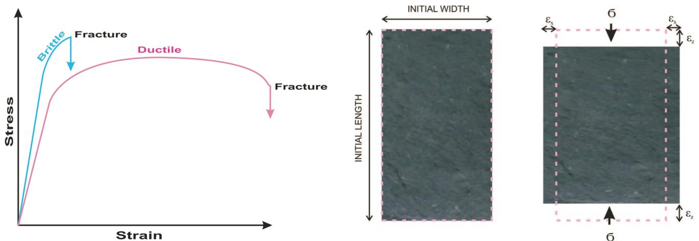
Fig. 1. A – Change of the rock sample dimensions under applied compressive stress. B – Graph showing two types of deformation that rock undergoes under applied stress. The blue curve is typical for brittle rocks while the pink one is typical for ductile rocks
