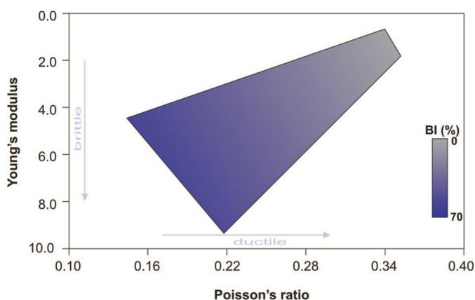
Fig. 2. Plot presenting the relationship between Young's modulus and Poisson's ratio for Brittleness Index (BI) estimation. The higher BI values the rock will be assumed to have, the more brittle and prone to generate artificial fractures network and therefore more efficient hydraulic fracturing will be [14] changed
