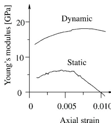
Fig. 3. Comparison of static and dynamic Young's modulus measured in triaxial tests of dry sandstones from the Red Wildmoor [6]
