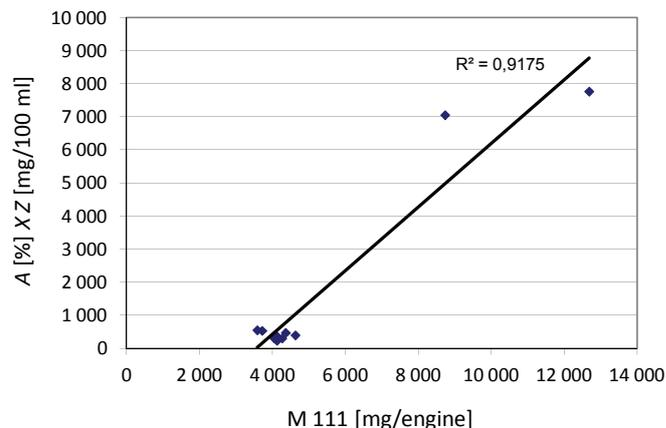
Fig. 4. Regression analysis ( $A \cdot Z$ ) versus the M 111 engine test results (without sample No. 3)
