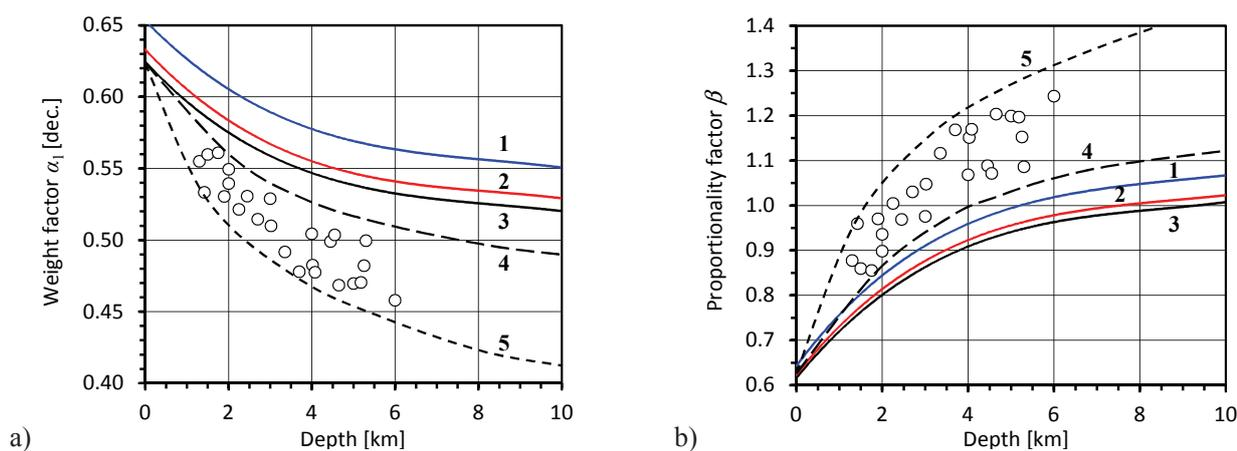
Fig. 4. Weight factor  $\alpha_i$  (a) and proportionality factor  $\beta$  (b) vs reservoir depth: 1 – dolomite, 2 – limestone, 3–5 – sandstone. Pressure gradient: 1–3 – 10 MPa/km, 4 – 13 MPa/km, 5 – 23 MPa/km; geothermal gradient – 30°C/km; ○ – examples of AHFP
