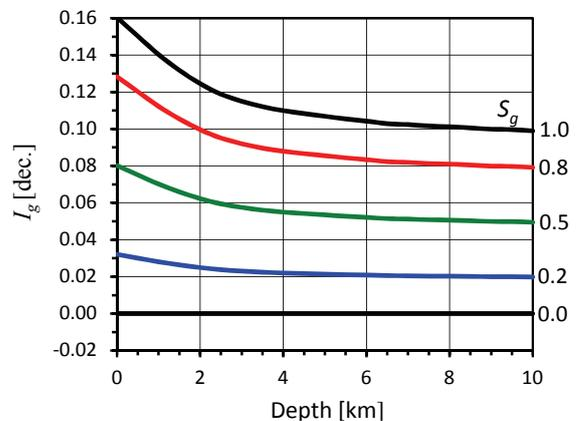
Fig. 3. Identification parameter vs depth for sandstone with  $\phi = 0.10$  at different gas saturation. Pressure gradient – 10 MPa/km, thermal gradient – 30°C/km
