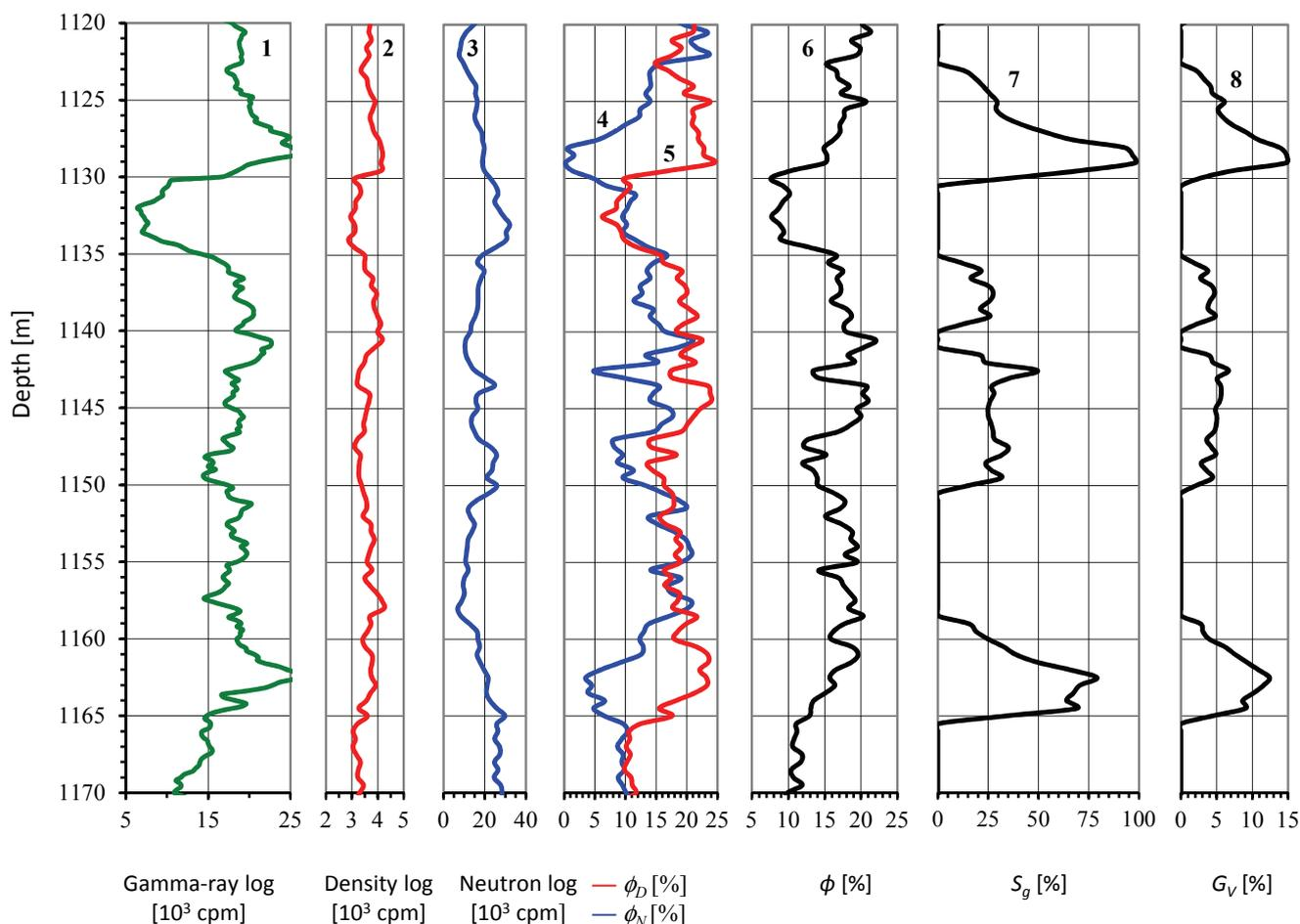
Fig. 5. Diagrams of radioactive logging in gas well (1 – gamma-ray log, 2 – density log, 3 – neutron log; cpm – counts per minute) and petrophysical parameters (4 – neutron porosity, 5 – density porosity, 6 – true porosity, 7 – gas saturation, 8 – volume gas content)
