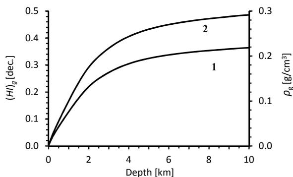
Fig. 1. Gas density  $\rho_g$  (1) and hydrogen index  $(HI)_g$  (2) vs depth. Pressure gradient – 10 MPa/km, thermal gradient – 30°C/km
