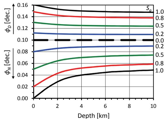
Fig. 2. Apparent porosities vs. depth for sandstone with  $\phi = 0.10$  at different gas saturation. Pressure gradient – 10 MPa/km, thermal gradient – 30°C/km
