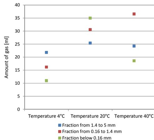
Fig. 2. Total amounts of released gas broken down into fractions and temperatures – brown coal [ml]
