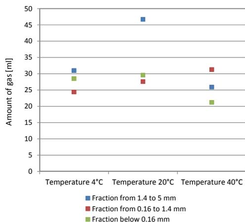
Fig. 1. Total amounts of released gas broken down into fractions and temperatures – hard coal [ml]
