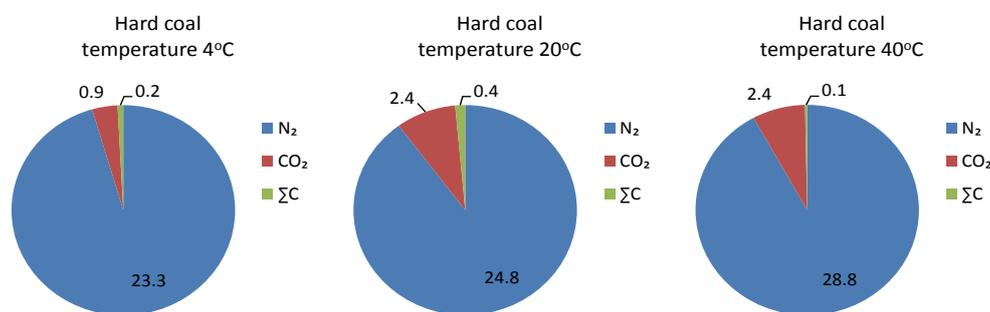
Fig. 3. Amounts of released nitrogen, carbon dioxide, and total hydrocarbons – hard coal, fraction from 0.16 to 1.4 mm [ml]
