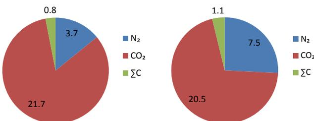
Fig. 8. Amounts of released nitrogen, carbon dioxide, and total hydrocarbons – brown coal [ml]
