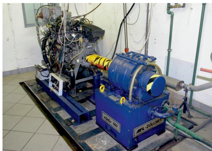
Fig. 2. A test stand with Peugeot DW10 engine according to the procedure CEC F-98-08 (INiG – PIB)
