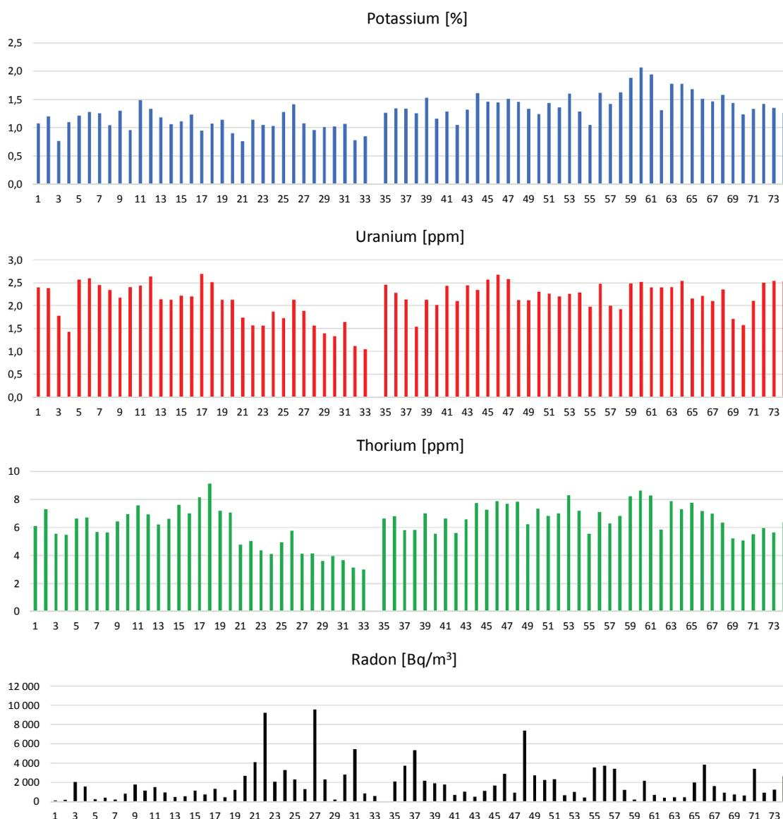
Fig. 5. Measured values for potassium, uranium, thorium, and radon along the Cergowa Mountain–Jasionka profile
