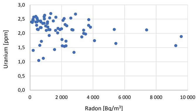
Fig. 6. Correlation graph of radon and uranium concentration measured in that same points in the field. Data collected in the Cergowa Mountain–Jasionka profile
