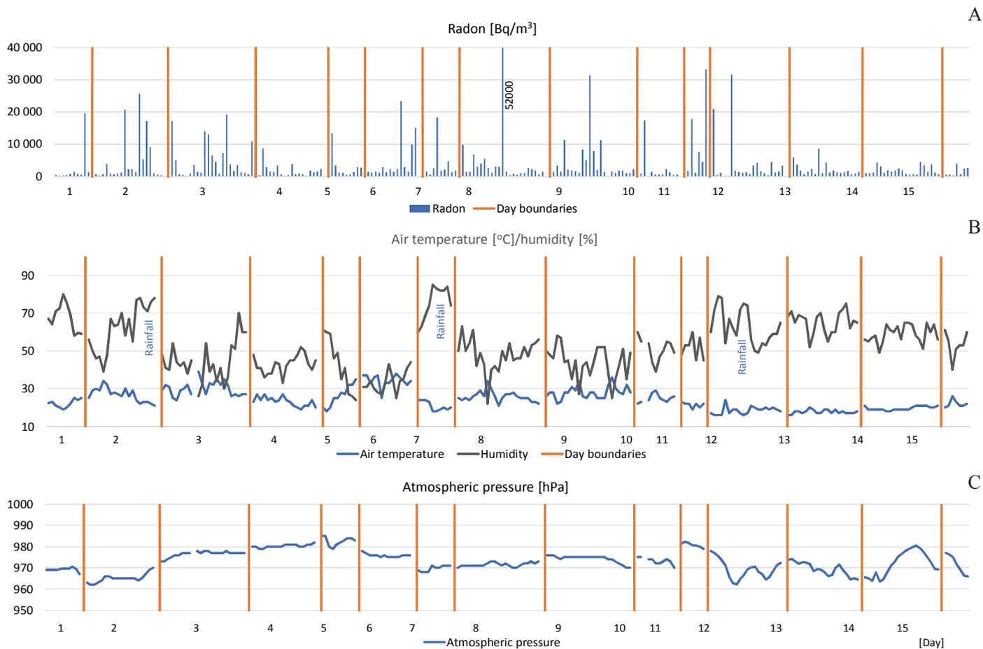
Fig. 3. Results of measurements: A – radon, B – air temperature and humidity, C – atmospheric pressure, during the 15 days of fieldwork
