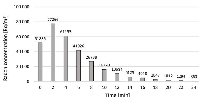
Fig. 2. Radon concentration graph, in function of time after the registration of a high concentration. Measurement was carried out during detection chamber purification
