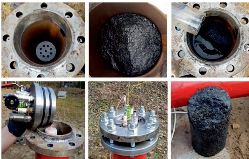
**Fig. 2.** Physical model of testing arrangement for gas fracturing of coal samples in laboratory scale: 1 – hard coal stabilizing steel sieve placed in the test system, 2 – coal cylinder placed on the sieve, 3 – flooding the system with water, 4 – closing the system with a plug with high-energetic fuel, 5 – closed test system, 6 – carbon cylinder after gas fracturing
