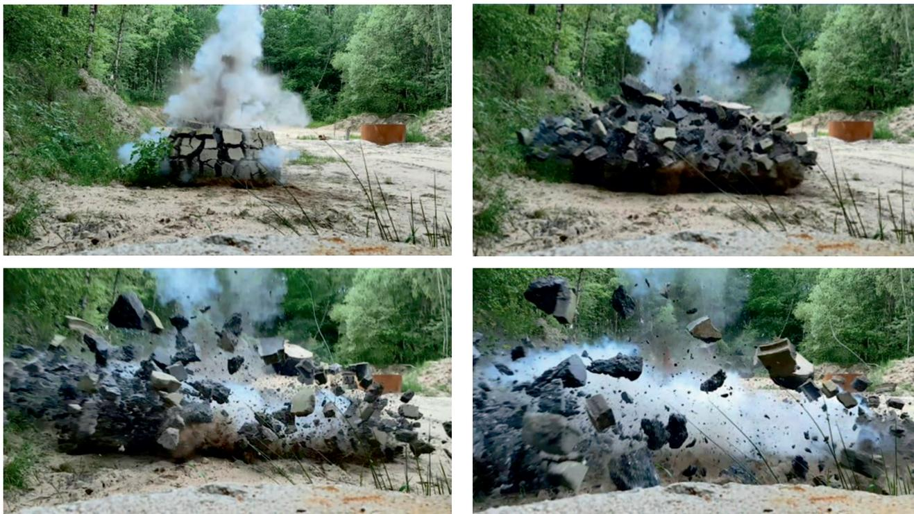
**Fig. 9.** The frames of the video from the shooting test No. 3 recording. Total damage and scattering of the concrete part is visible. The steel pipes remain in good condition, enabling free assessment of cumulative cuts. However, lack of undisturbed concrete body excludes possibility of target penetration depth measurement
