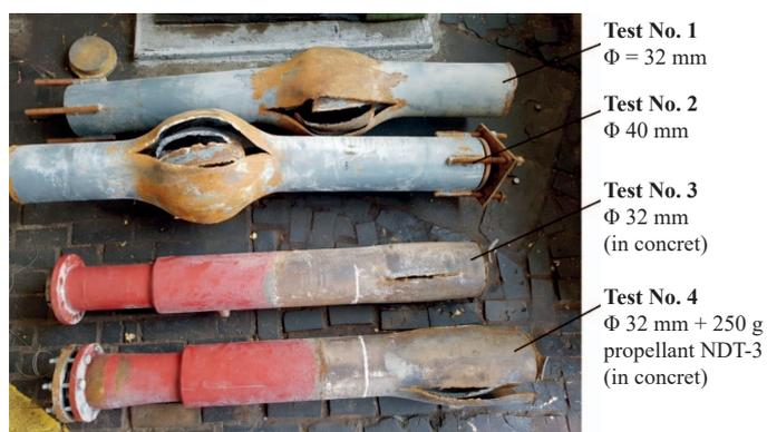
**Fig. 14.** Statement of shooting models, on which tests of multi-layered target perforation were completed
