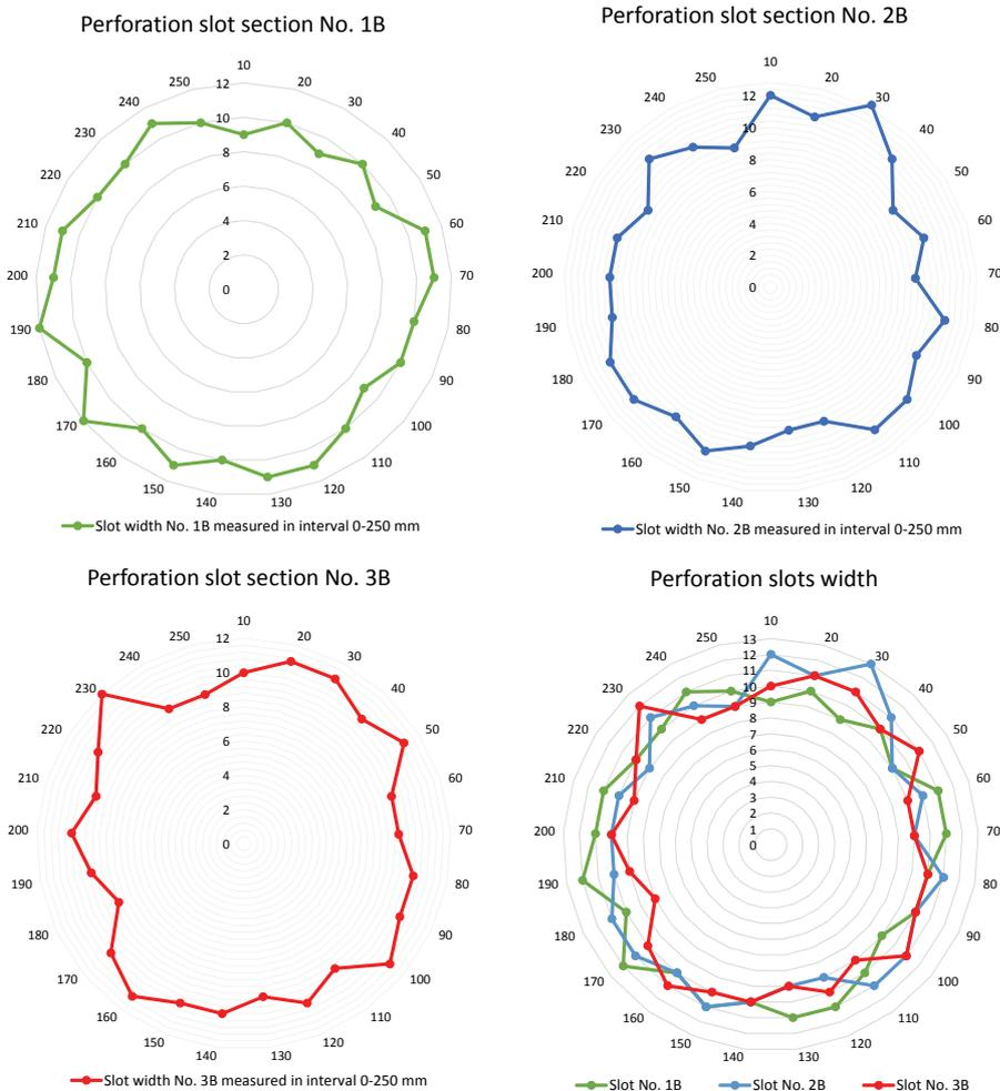
**Fig. 12.** Statement of widths for the cumulative slots created within the body pipe of the tool ( $\varnothing = 5''$ ), created by firing linear shaped charges of  $\varnothing = 32$  mm diameter and  $L = 250$  mm length, jointly with NDT-3 propellant of 250 g total mass
