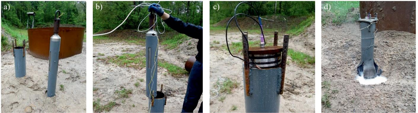
**Fig. 2.** View of tested device model on the fire-ground; a)  $\varnothing = 7''$  casing pipe, b) conceptual fracperforator being run down the shooting model by means of the cap and wireline, c) movable plug with current pass-through d) the view after the linear shaped charges were fired
