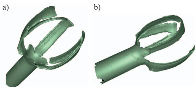
**Fig. 5.** The result of three-dimensional scanning of body pipe of the tool removed from inside of shooting model
