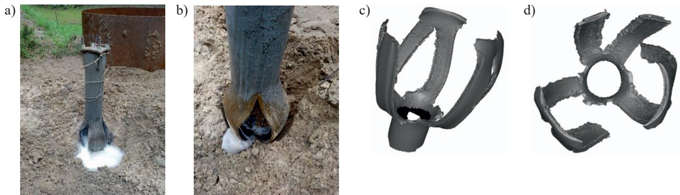
**Fig. 3.** A view of shooting model following the test completion; a) front view, b) side view, c) d) the views of 3D scans of tested tool body pipes, removed from inside of the shooting model
