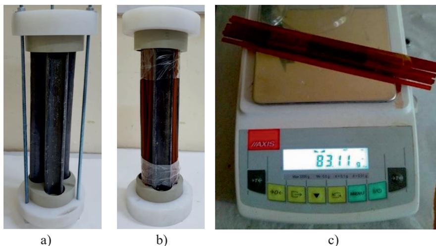
**Fig. 10.** View of the working part of the tested arrangement; a) test version without propellant; b) view of target, internal part of the tool with the linear shaped charges surrounded by the NDT-3 propellant; c) moment of weighing the NDT-3 propellant intended for fracperforator model arming; the tested arrangement was armed with homogeneous propellant in the form of three bundles of tubular propellant, each having 83 g mass on average. The total mass of the propellant did not exceed 250 g
