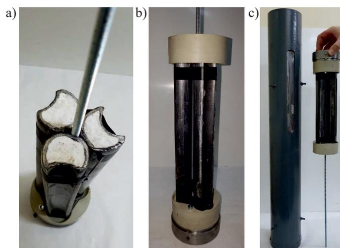
**Fig. 1.** A – view of three linear shaped charges, seated in lower centraliser seat; B – view of complete perforating arrangement, equipped with centralisers, carrying rod and steel cover of the head; C – view of fracperforator model, prepared for fire-ground testing of multi-layer target perforation
