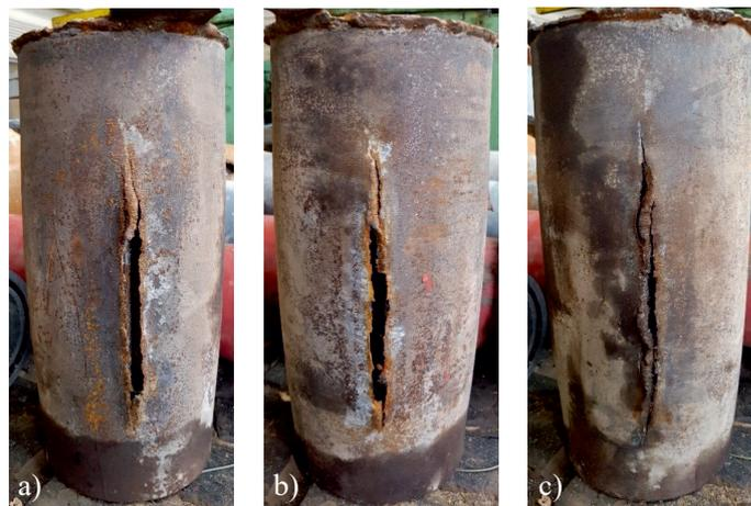
**Fig. 11.** View of casing pipe, perforated with linear shaped charges of  $\varnothing = 32$  mm diameter,  $L = 250$  mm length, in set-up with 250 g NDT-3 propellant
