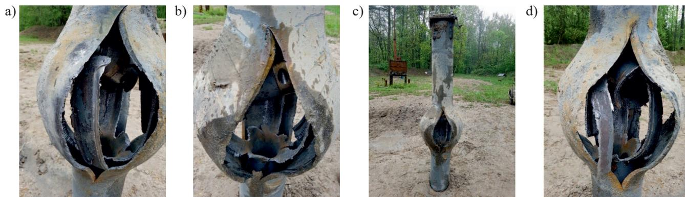
**Fig. 4.** View of various perspectives of perforated body and casing pipe in shooting test No. 2, performed with use of the linear shaped charges of  $\varnothing = 40$  mm diameter and  $L = 250$  mm length
