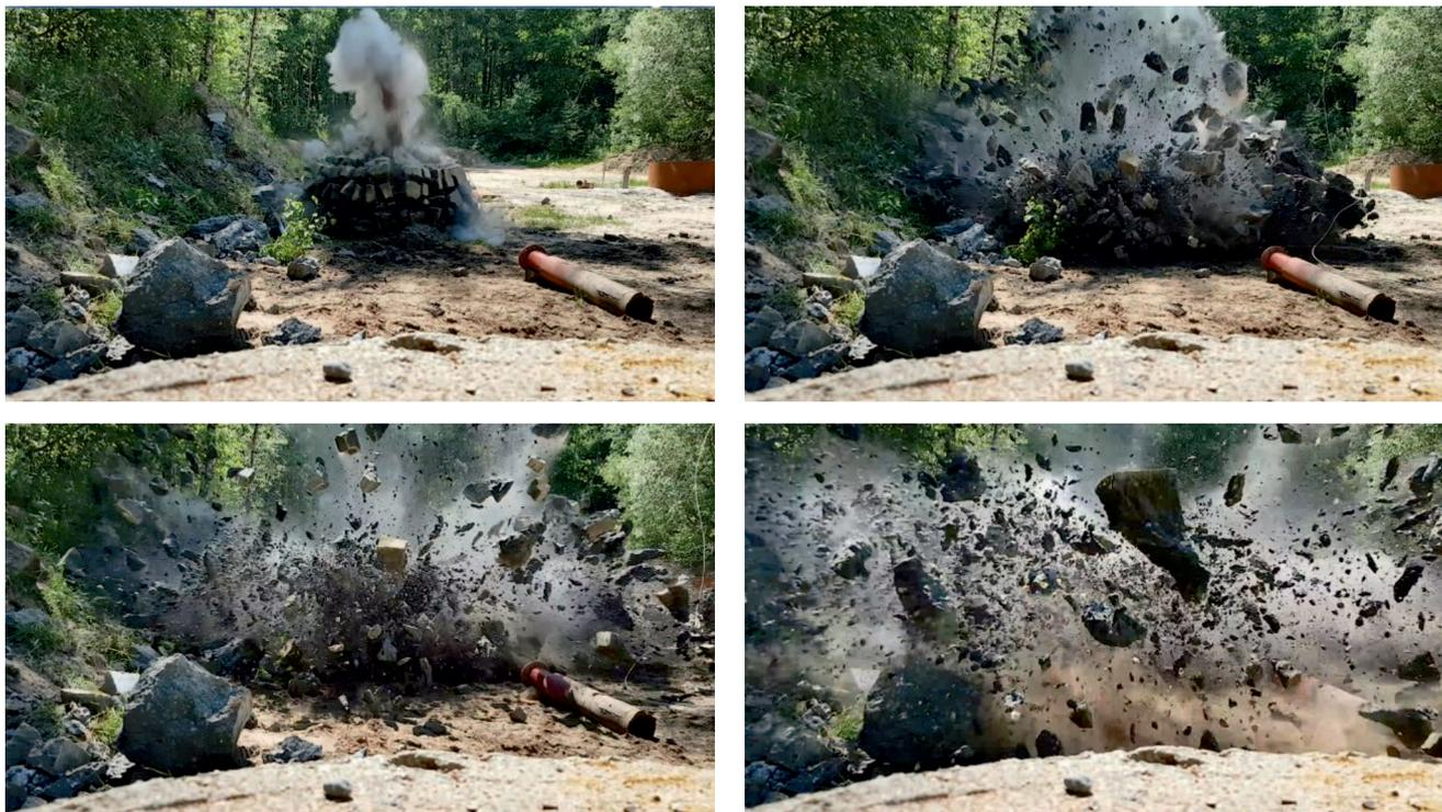
**Fig. 13.** Video images from the shooting test No. 4 recording. Total damage and scattering of the concrete part is visible. The steel pipes remain in good condition, enabling the free assessment of cumulative cuts. However, the lack of undisturbed concrete body excludes possibility of target penetration depth measurement
