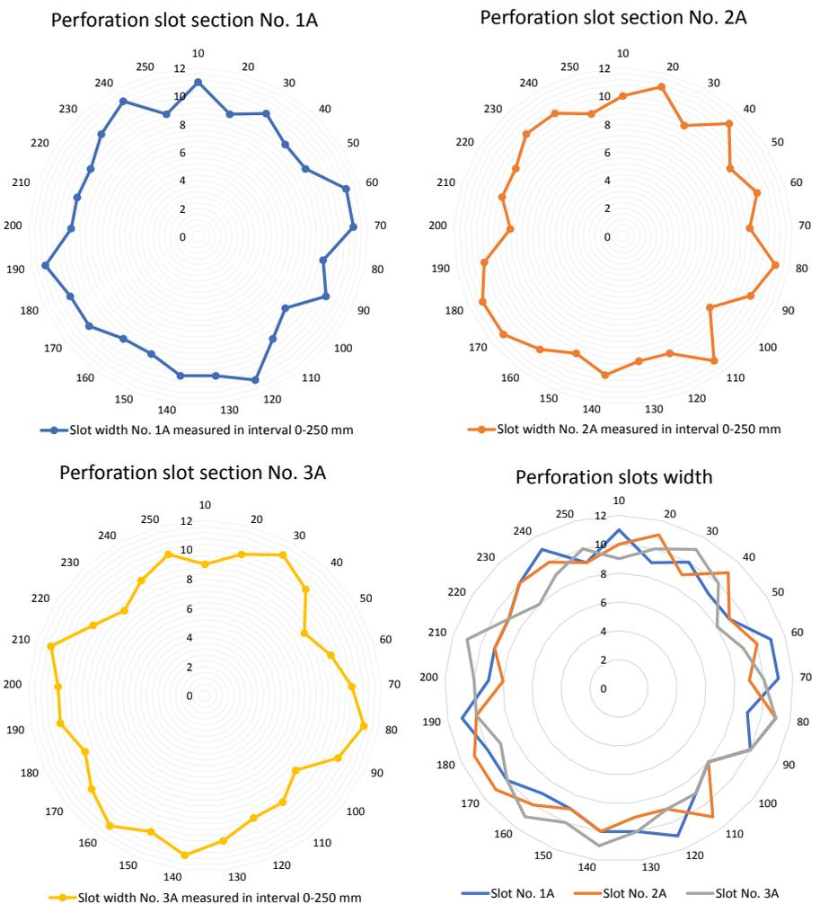
**Fig. 8.** Statement of widths for cumulative slots created within body pipe of the tool ( $\varnothing = 5''$ ) in result of firing linear shaped charges of  $\varnothing = 32$  mm diameter and  $L = 250$  mm length
