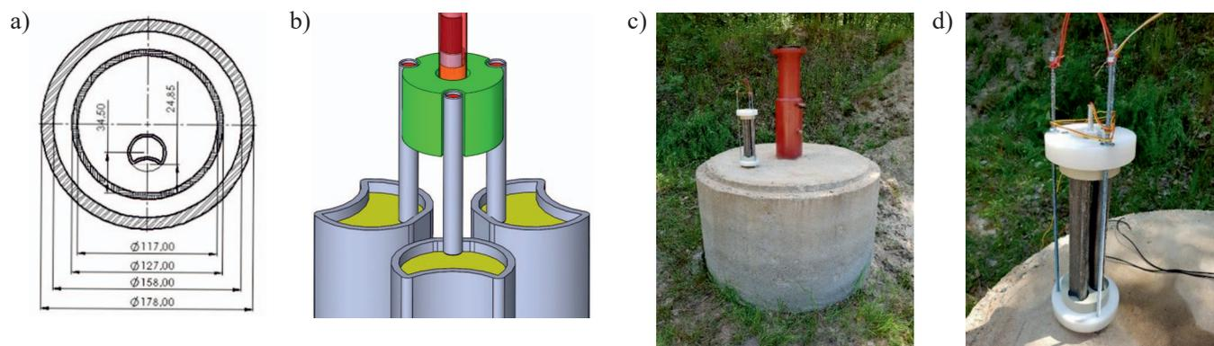
**Fig. 6.** View of test arrangement for realisation of multi-layer perforation with linear shaped charges, a) cross sectional view of shooting stand with marked position of single charge; b) design of ballistic line path; c) the concrete and steel stand; d) the key elements of the testing arrangement – three linear shaped charges united with a system of centralisers; firing unit; temporary carrying system
