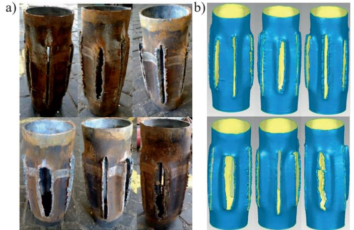
**Fig. 7.** View of body pipe  $\varnothing = 5''$ , removed from casing pipe after completion of the test (left side); results of 3D scanning of the same body pipe
