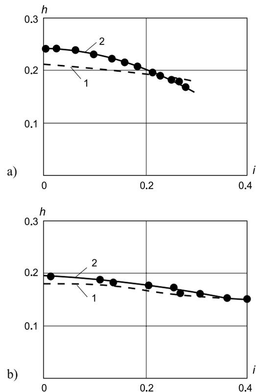
**Fig. 4.** Theoretical (1) and experimental (2) pressure characteristics of the jet pump for different values of the geometric parameter  $K_p = 5.012$  (a);  $K_p = 6.464$  (b)
