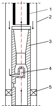
**Fig. 1.** Schematic diagram of the borehole ejection system: 1 – tubing string; 2 – borehole wall; 3 – mixing chamber and diffuser; 4 – working nozzle; 5 – packer
