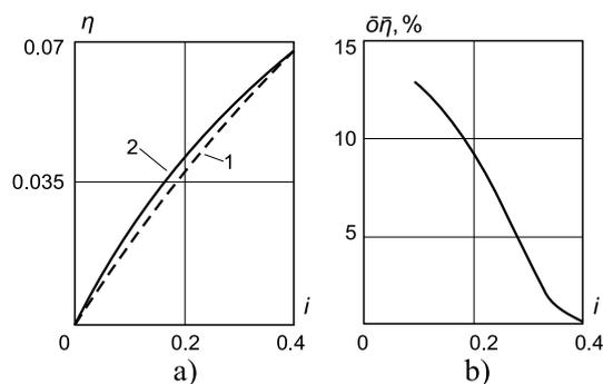
**Fig. 5.** Comparison of energy characteristics of the jet pump: a) theoretical (1) and experimental (2) dependences of the efficiency on the injection coefficient; b) relative error of theoretical and experimental values of efficiency
