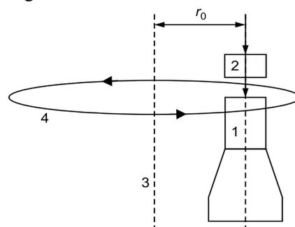
**Fig. 2.** Asymmetric swirling of the injected flow: 1 – mixing chamber and diffuser; 2 – working nozzle; 3 – axis of the well; 4 – trajectory of the liquid particles
