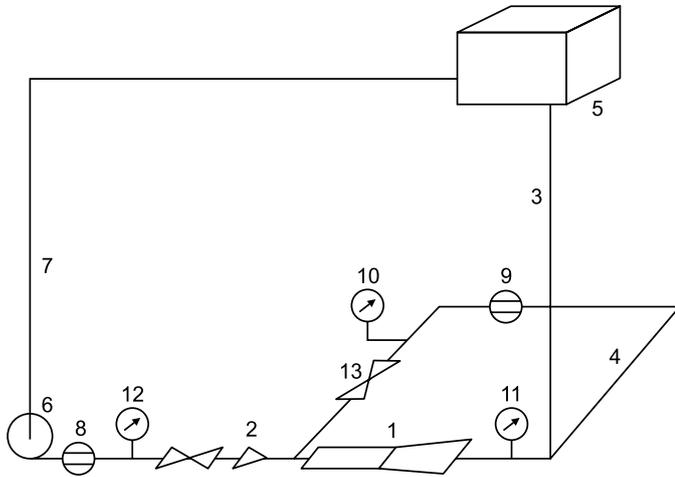
**Fig. 3.** Laboratory setup for investigating the operating process of a jet pump in conditions of swirling injected flow (description in the text)
