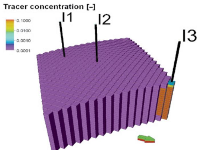
**Fig. 14.** Scenarios of Option I. Initial iteration. The concentration of the tracer injected with the I3 well
