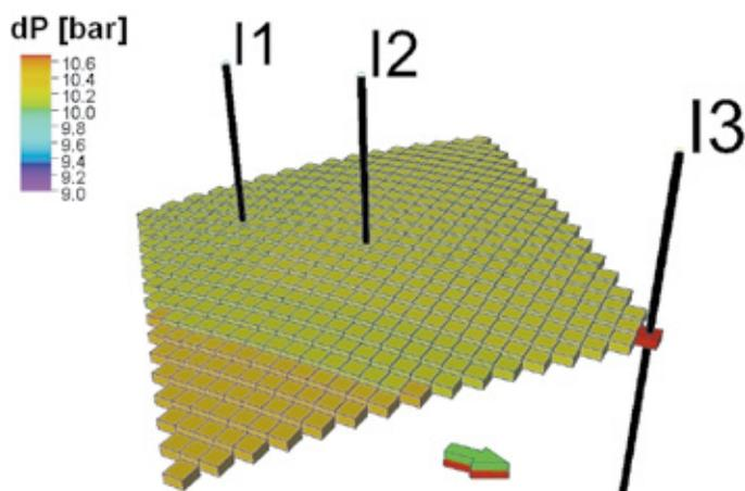
**Fig. 13.** Scenarios of Option I. Initial iteration. Pressure steps across the top boundary of the reservoir
