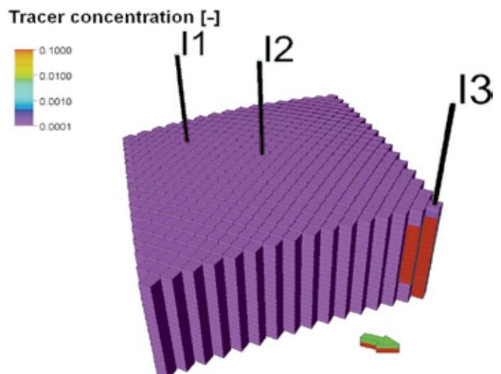
Fig. 19. Scenarios of Option II. Initial iteration. The concentration of the tracer injected with the I3 well
