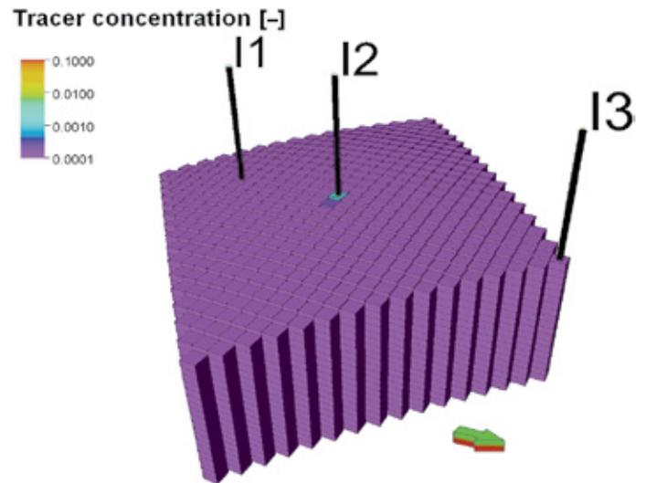
Fig. 18. Scenarios of Option II. Initial iteration. The concentration of the tracer injected with the I2 well
