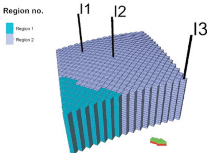
**Fig. 4.** Definition of regions for the leakage beyond the structural trap boundary of the reservoir: region no. 1 – external zone, region no. 2 – internal zone. View of reservoir layers only ( $k = 2 - 20$ )
