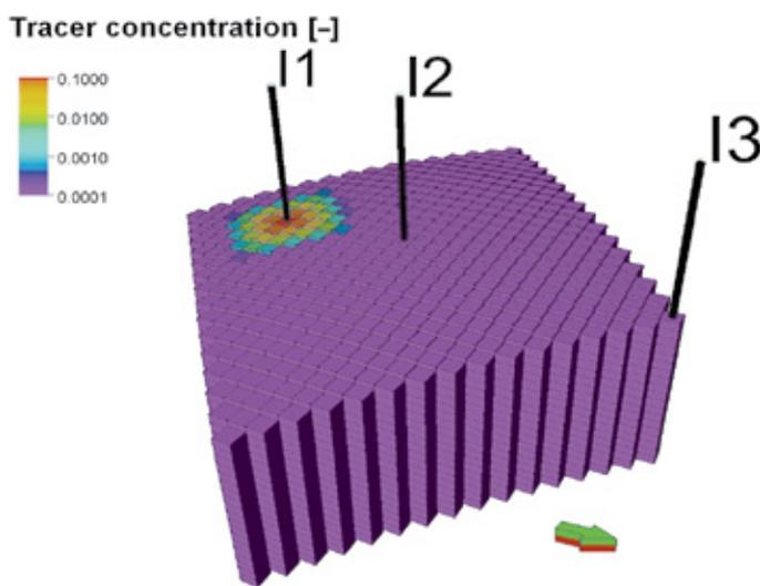
Fig. 17. Scenarios of Option II. Initial iteration. The concentration of the tracer injected with the I1 well
