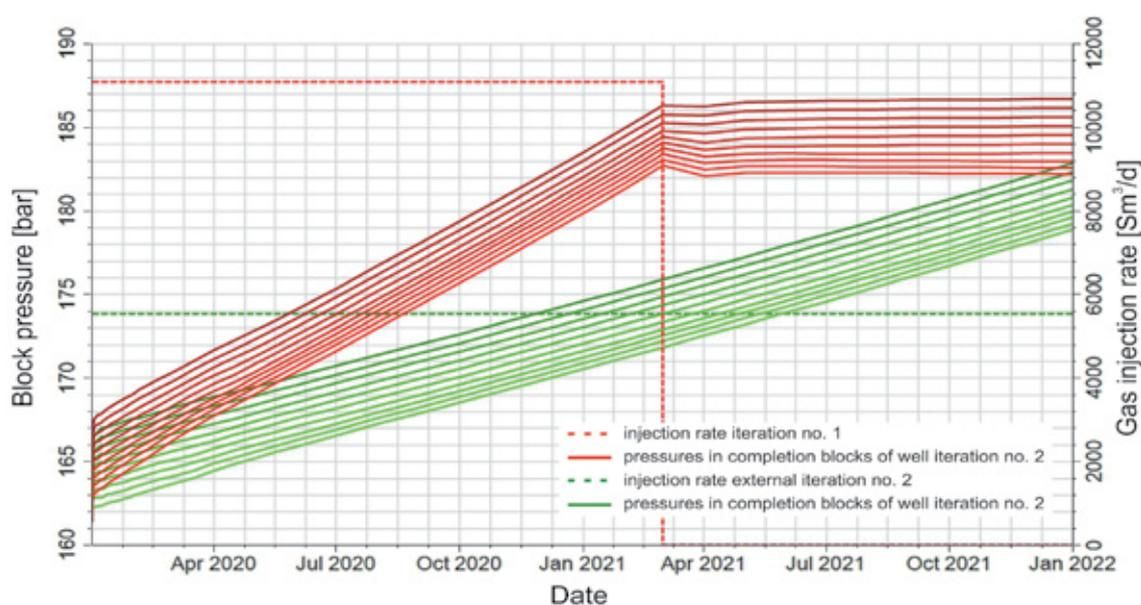
**Fig. 15.** Scenarios of Option II. Initial iteration (red lines): CO<sub>2</sub> injection rate of I3 well (dashed red line), pressure in blocks of I3 well completion (solid red lines); iteration with reduced injection rate (green lines) CO<sub>2</sub> injection rate of I3 well (dashed green line), pressure in blocks of I3 well completion (solid green lines)
