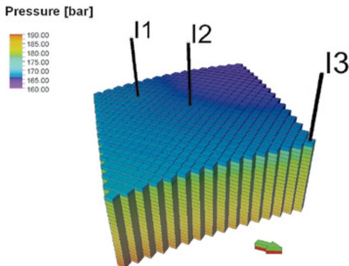
**Fig. 3.** Initial pressure distribution. Overburden layer,  $k = 1$ , reservoir layers,  $k = 2 - 20$
