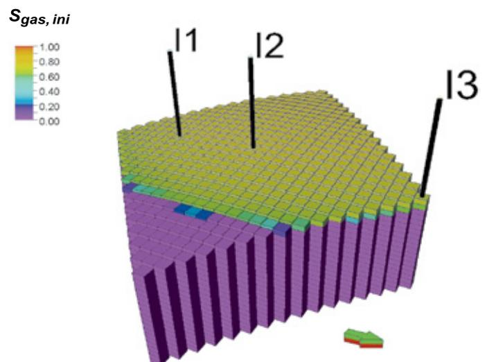
**Fig. 2.** Initial gas saturation distribution. Reservoir layers only ( $k = 2 - 20$ )
