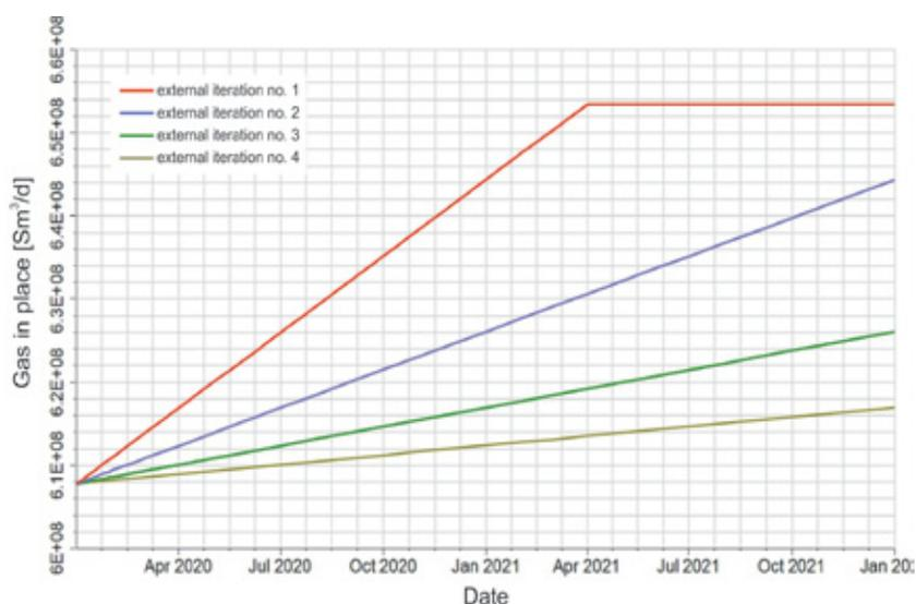
**Fig. 10.** Scenarios of Option II. Sequestration capacity for subsequent iterations
