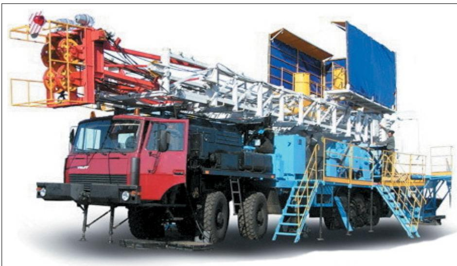
**Figure 1.** Truck mounted repair-drilling rig ARB-100
