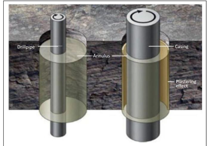
Figure 1. The effect of mechanical clogging during drilling on casing (comparison: conventional pipes on the left/casing pipes on the right) (Courtesy of Schlumberger Comp.)
