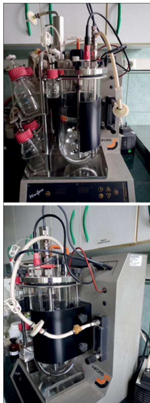
**Figure 6.** Bioreactor used for bacterial suspension preparation for the purpose of biocide testing
