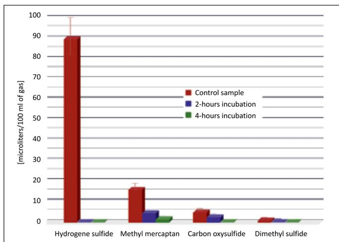
**Figure 1.** Example diagram showing the results of incubating the tested samples; the content of sulphur compounds in the gas tend to decrease after adding an H<sub>2</sub>S scavenger, based on a triazine derivative
