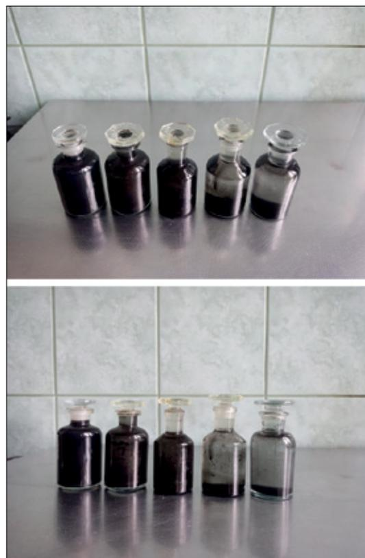
**Figure 3.** The incubation of sulphate reducing bacteria (anaerobes) isolated from formation waters of underground gas storage facilities. The photos show a 30-day incubation in a liquid medium
