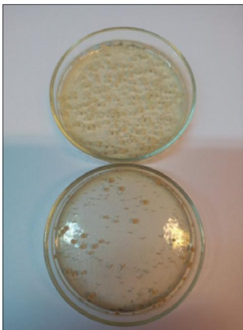
**Figure 4.** Colonies of aerobic bacteria isolated from polymer drilling mud
