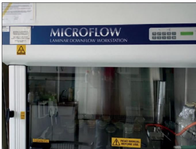
**Figure 7.** Laminar workstation with air downflow used to study biological material under sterile conditions
