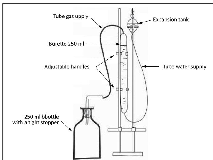
**Figure 2.** Laboratory equipment for biocide testing using the degasation method
