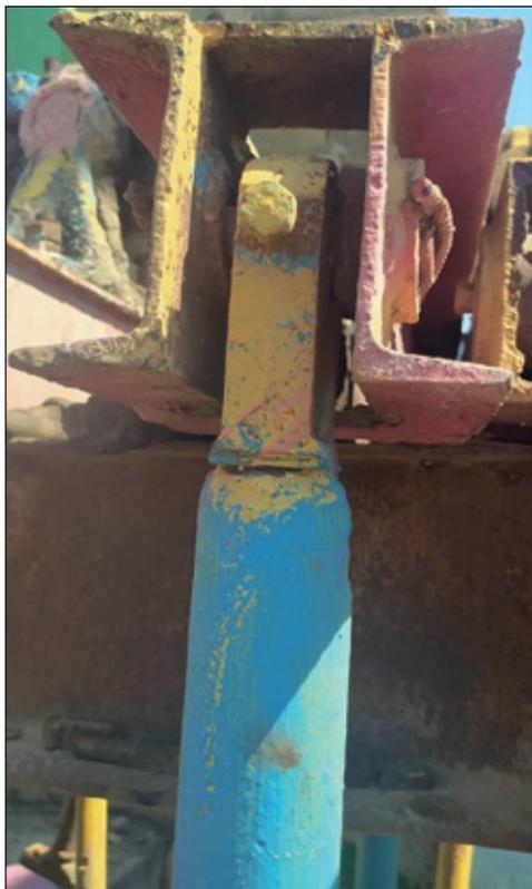
**Figure 9.** Deformation and wear of the connecting rod-traverse connection
