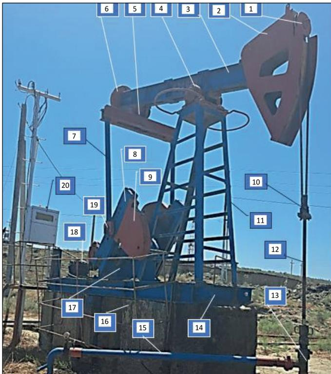
**Figure 2.** General view of the converting mechanism – pump jack: 1 – block for rope suspension; 2 – the head of the balancer; 3 – balancer; 4 – support; 5 – traverse; 6 – equalizing weight; 7 – connecting rod; 8 – crank; 9 – counterweight; 10 – suspension point of the rod string; 11 – rack; 12 – polished stem; 13 – tee; 14 – frame; 15 – flow line; 16 – concrete foundation; 17 – reducer; 18 – electric motor with V-belt transmission; 19 – brake; 20 – control station
