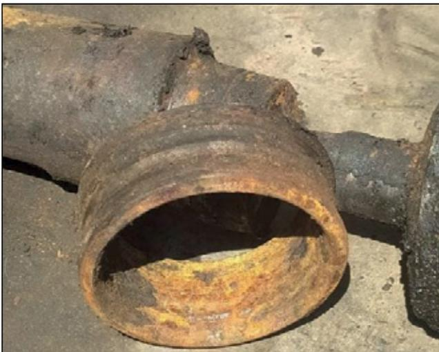
**Figure 11.** Bottom support of the connecting rod
