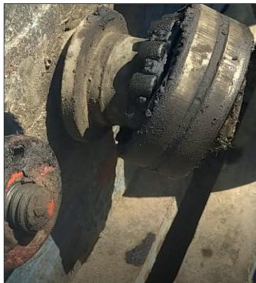
**Figure 5.** Damaged crank support due to vibrations
