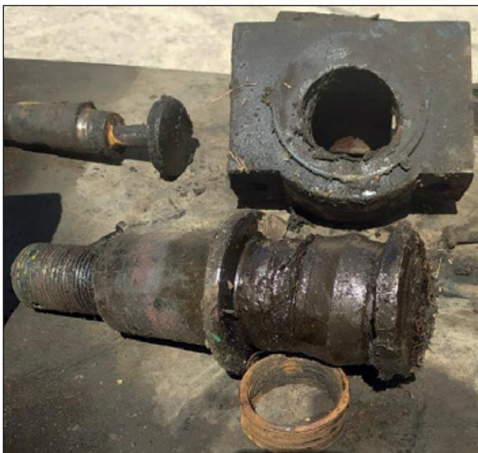
**Figure 10.** Connecting rod pin wear
