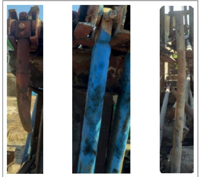
**Figure 7.** Deformation and fracture of connecting rods
