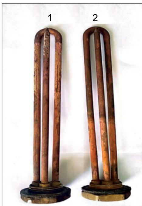
**Figure 4.** Heating element of the heating boiler: 1 – heating element working without magnetic field, 2 – heating element working with magnetic field
